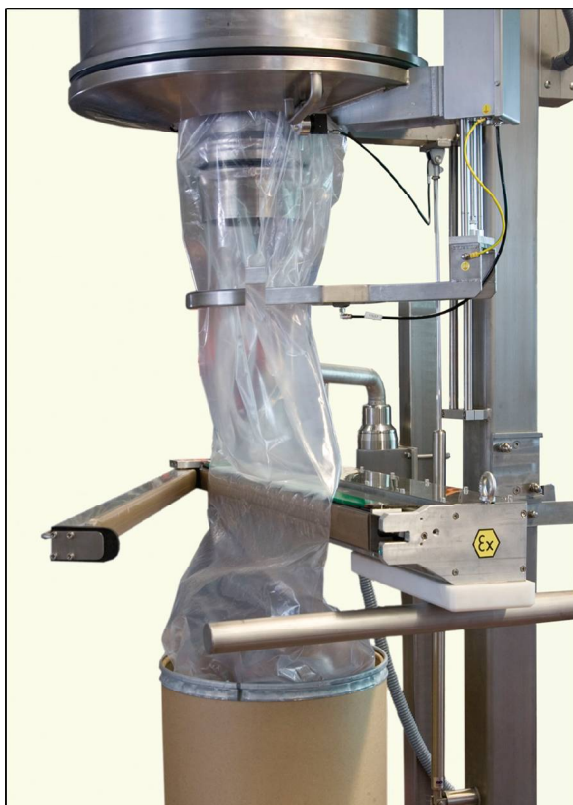
Continuous liner system with welding machine
