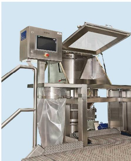
If the production batch is finished, the operator starts the automatic cleaning and drying process by using the touch panel. The entire system is completely automatically CIP cleaned, and then dried with conditioned hot air. One CIP cleaning and drying cycle lasts, depending upon the product and degree of contamination, about 60 minutes. Follow-on manual cleaning is not necessary.
