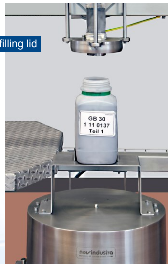
General view with carrying frame, product hopper, dosing channel, scale with mounted lifting lifting device and control system.
