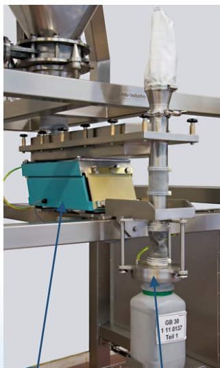
General view with carrying frame, product hopper, dosing channel, scale with mounted lifting lifting device and control system.
