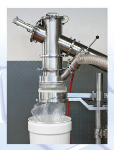
Dosing Screw with Filling head, pre-filter and sealing ring
