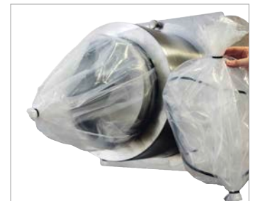
Cut the liner and dispose of the removed product
